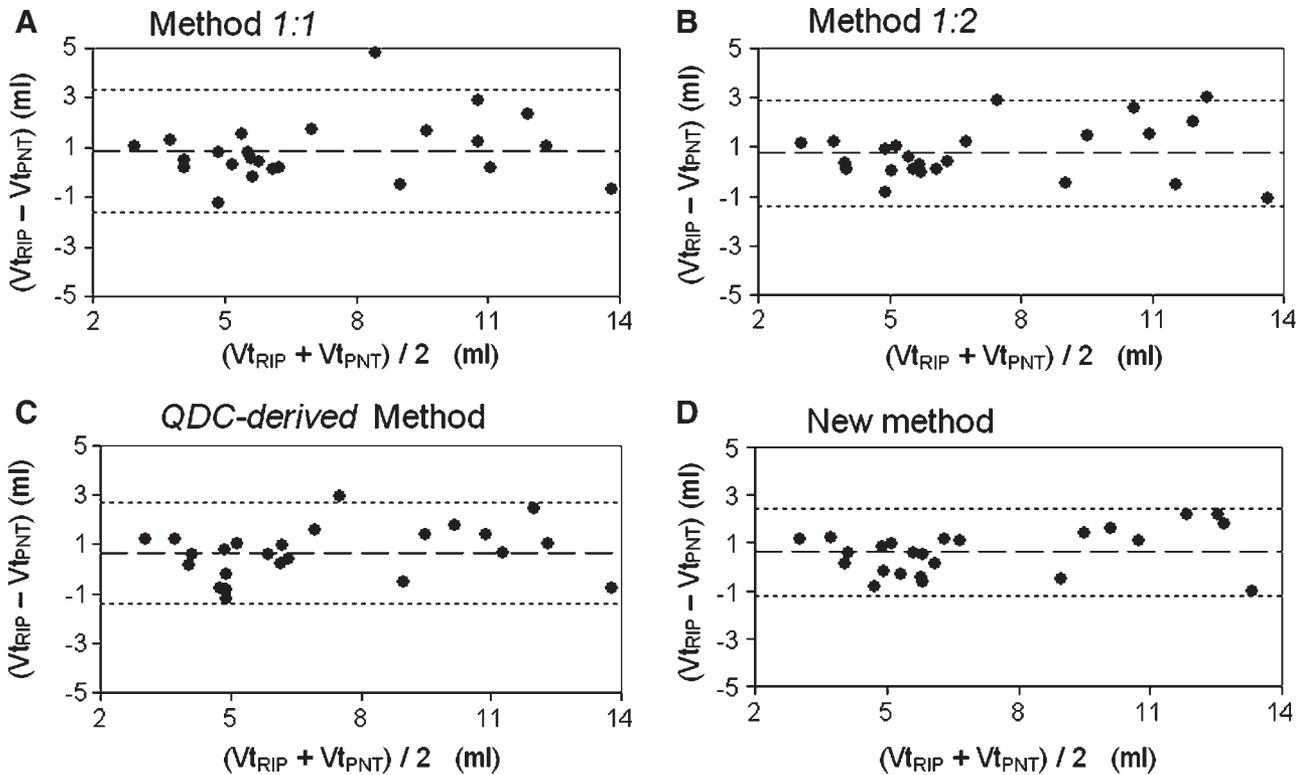
**Fig. 3. Bland-Altman plots of the differences between mean VT<sub>PNT</sub> and mean VT<sub>RIP</sub> calculated with method 1:1 (A), method 1:2 (B), QDC-derived method (C), and the new method (D). Central and lateral dotted lines represent mean differences and the limits of agreement respectively.**
